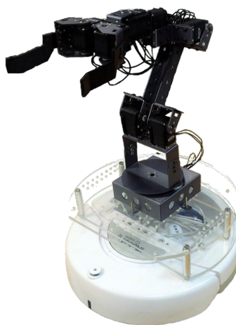
Figure A.1: Little John, a nonholonomic mobile manipulator (courtesy of MACRO Research Group).
